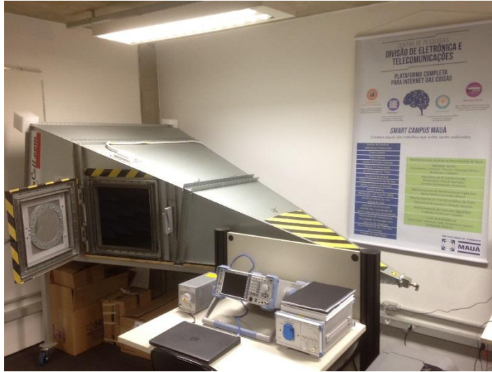
Figura 1: 5405 GTEM! Test Cell instalada na Sala R401
